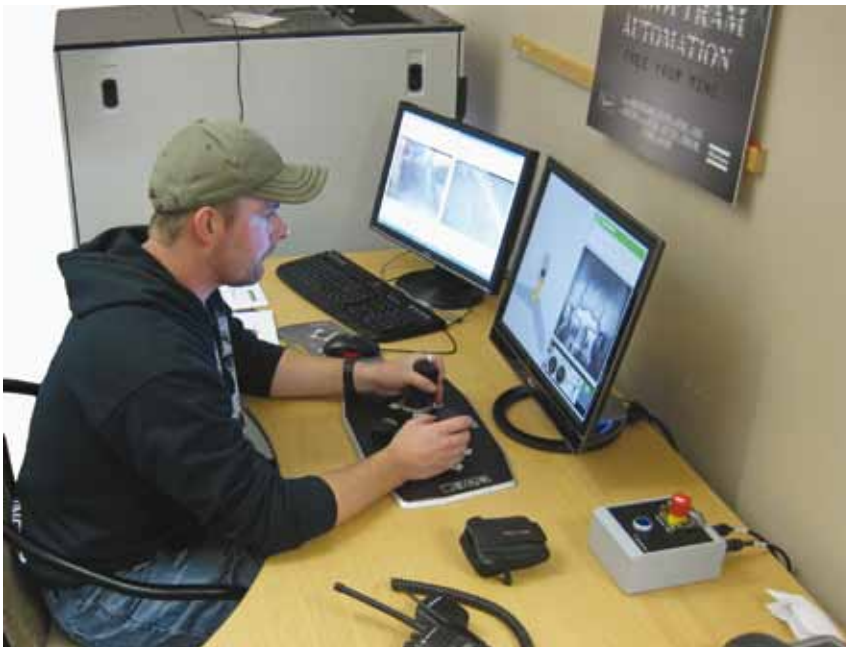
To demonstrate, Diavik set up a control centre in the mine's main accommodations. From surface, Diavik Underground Services Engineer Chris Pichurski with video display and controls, operates the scooptram remotely.
