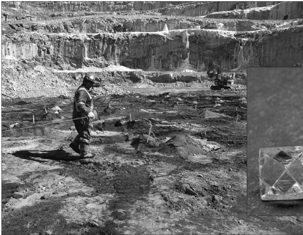
Blaster Roger Lirette ties in a blast pattern in the Diavik A154 open pit.
